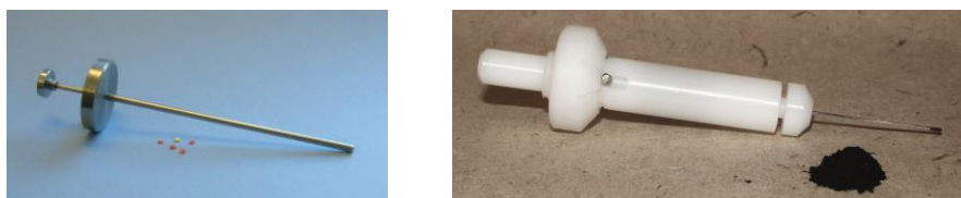
Figure 3. Sample handlers for e.g. paper and powder.
